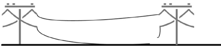
Figure 2: Downed Broken Conductor
